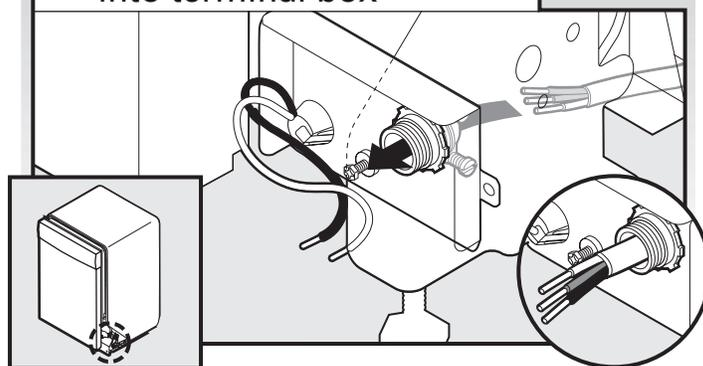
Route cable so that it does not touch dishwasher motor or lower part of dishwasher tub. Pull cable through cable clamp in terminal box.
